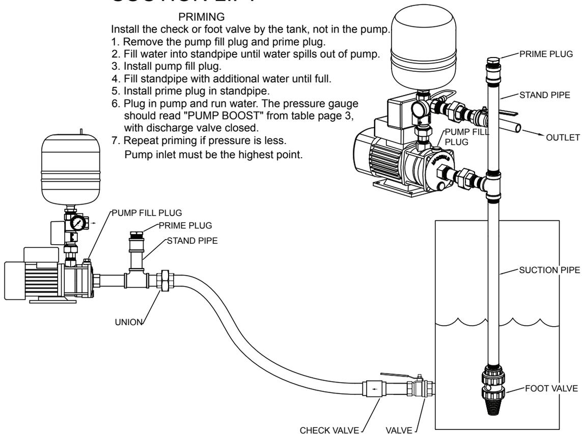
The pump inlet must also be the highest point. There can be no humps in the line as shown here:
