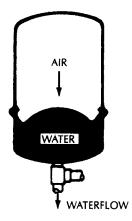
Water is being drawn from the tank: Compressed air in the tank forces water out.
