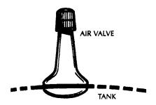
3. If the air pressure is below the cut-in setting, add air to the tank. Use an air compressor or a portable air storage tank to increase the air pressure to be 2 P.S.I. below the pump pressure switch cut-in setting. Raise the pressure slowly, checking it periodically with an accurate tire pressure gauge, until the desired pressure is reached.
