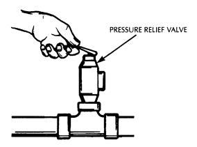
If after manually operating the valve it fails to completely reset and continues to release water, immediately shut off the pump and open a cold water faucet to drain the water out of the water tank and piping. Then replace the pressure relief valve with a new one (rated at 100 P.S.I. max.).
