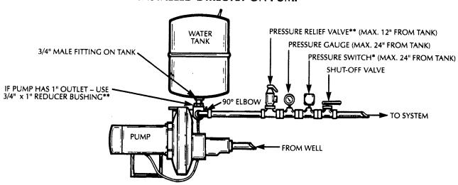
NOTES: \*OPTIONAL...MUST BE INSTALLED IF PUMP DOES NOT HAVE A PRESSURE SWITCH \*\*NOT FURNISHED...MUST BE PURCHASED LOCALLY.
