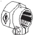
The A.Y. McDonald Mac-Pak compression system is a simple, convenient method of connection for lead pipe.
